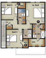
construction cost. All the floor framing runs in the same direction for the entire house, and it bears upon a wall running through the center of the home. The minimal breaks in the plan occur only on the front elevation to create breaks in the massing. This home is illustrated with both mid-century modern and Craftsman elevations to show the varied looks that can be achieved with the same floor plan.
