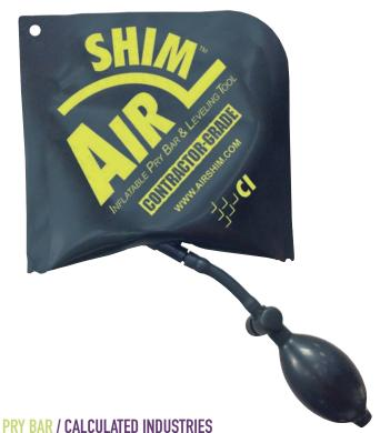
The inflatable pry bar and leveling tool is powerful enough to raise 300 pounds yet so soft it won't scratch surfaces. The easy-to-squeeze hand pump enables a lone user to lift, shift, align, level, plumb, adjust, or just hold materials, windows, doors, or heavy appliances still without assistance from shims, wedges, or a second pair of hands. AirShim measures 6 inches by 6½ inches on its sides, by about 1/16-inch high when deflated and 21/2 inches high when inflated.
