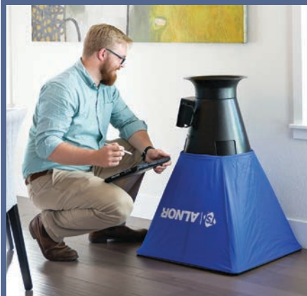
Nathan Kahre gets a readout from a capture hood, used to measure air coming out of a vent, and to double-check HVAC installations.
